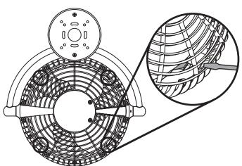
Release the nut by hand to take off the blade.
